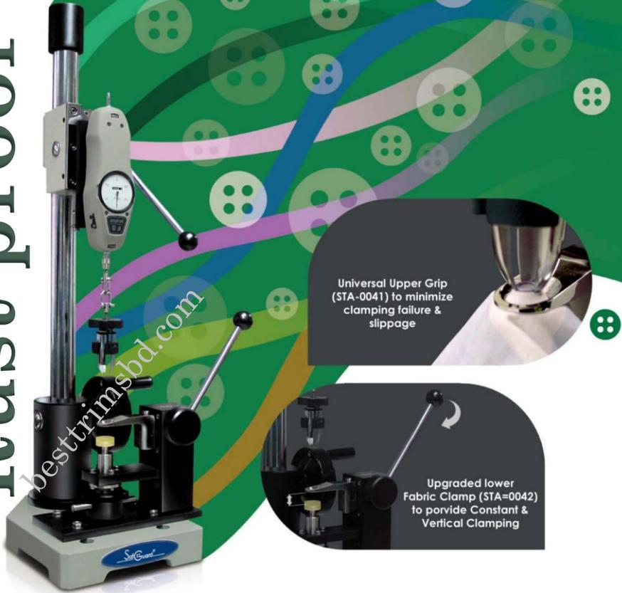
Universal Upper Grip (STA-0041) to minimize clamping failure & slippage
